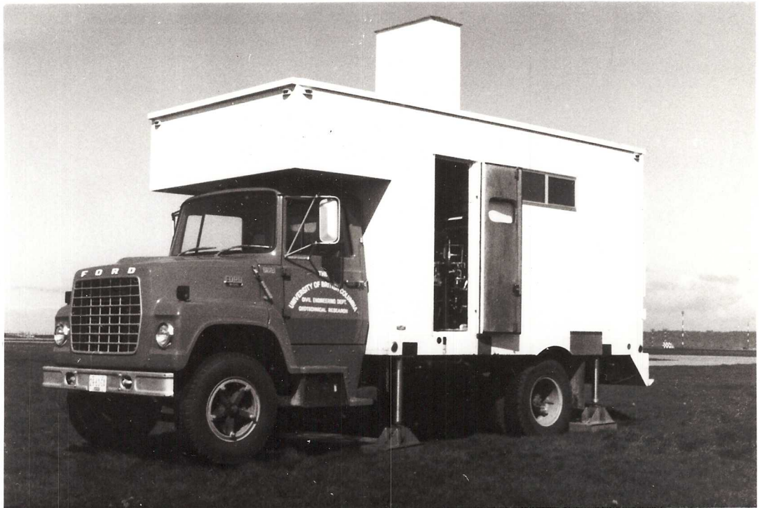
FIG.1 - UBC Field Research Vehicle, supported and leveled on large pads, raised mast houses penetration device.
